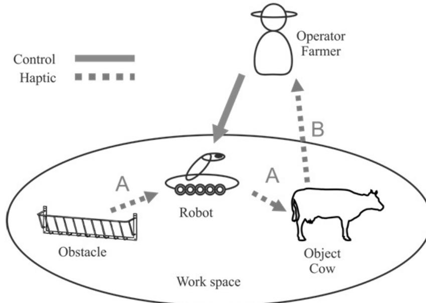
Fig. 1. Relationships between mobile robot, operator and obstacle over course of control using haptic device: A – direct interaction; B – indirect interaction
