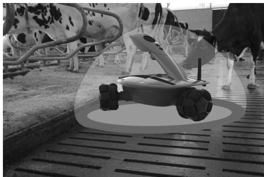
Fig. 5. Combining image from mobile robot's camera with computer-generated image
